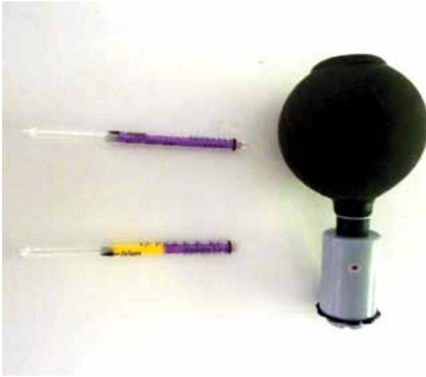
Figure 1.7. Dräger tubes specifically for acetic acid and pump to draw out air. The upper tube shows negative for acetic acid, while the lower shows positive (indicator turns yellow).
