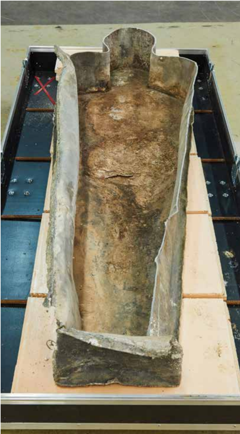
Figure 1.5. Example of preferential degradation at the base of a seventeenth-century lead sarcophagus due to the action of body decomposition fluids.
